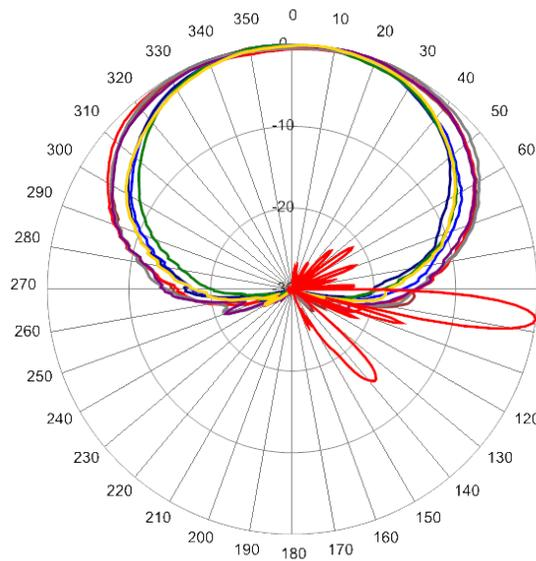
3500 MHz Azimuth with Elevation 7° Single Column
