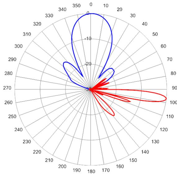
3500 MHz Azimuth 0° with Elevation 7° Service Beam
