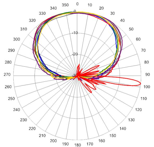
3920 MHz Azimuth with Elevation 7° Single Column
