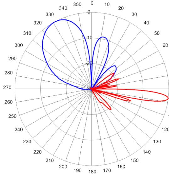
3500 MHz Azimuth 30° with Elevation 7° Service Beam
