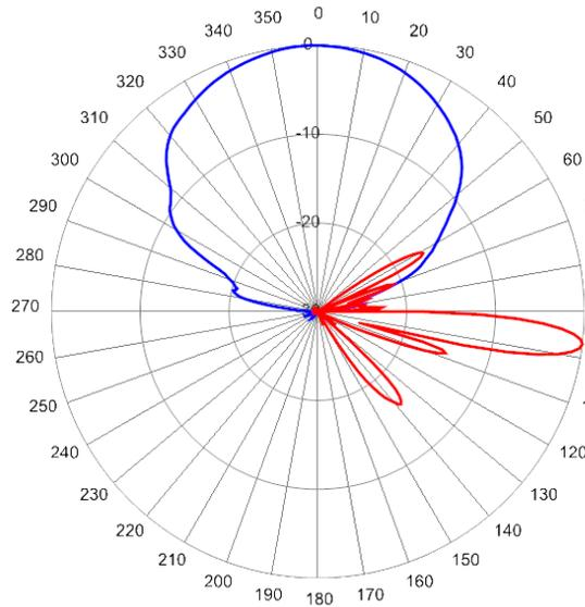
3500 MHz Azimuth with Elevation 7° Broadcast Beam
