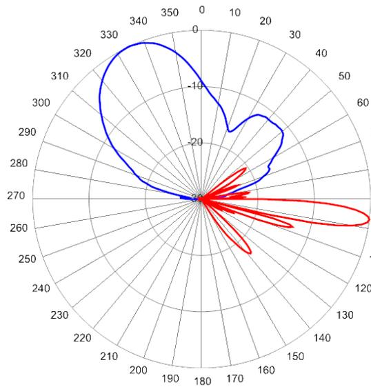
3500 MHz Azimuth with Elevation 7° Soft Split
