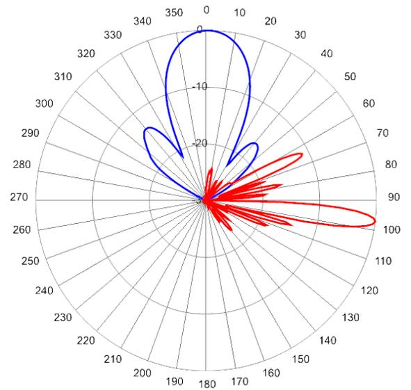
3920 MHz Azimuth 0° with Elevation 7° Service Beam
