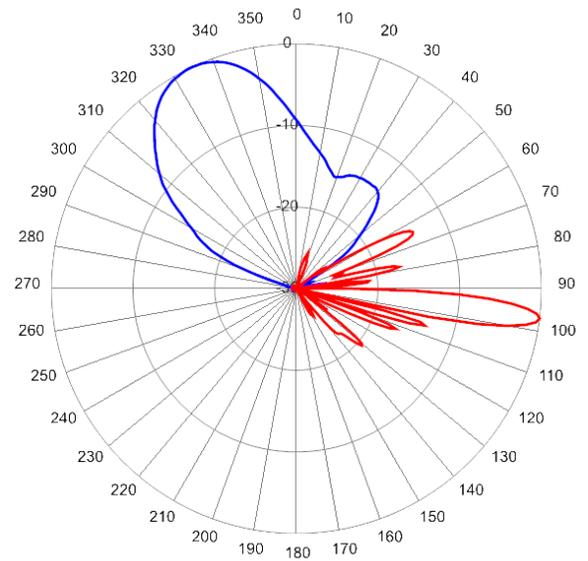
3920 MHz Azimuth with Elevation 7° Soft Split
