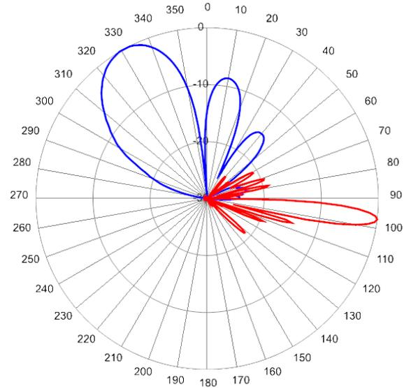
3820 MHz Azimuth 30° with Elevation 7° Service Beam
