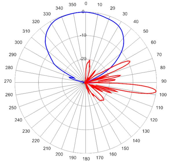
3920 MHz Azimuth with Elevation 7° Broadcast Beam
