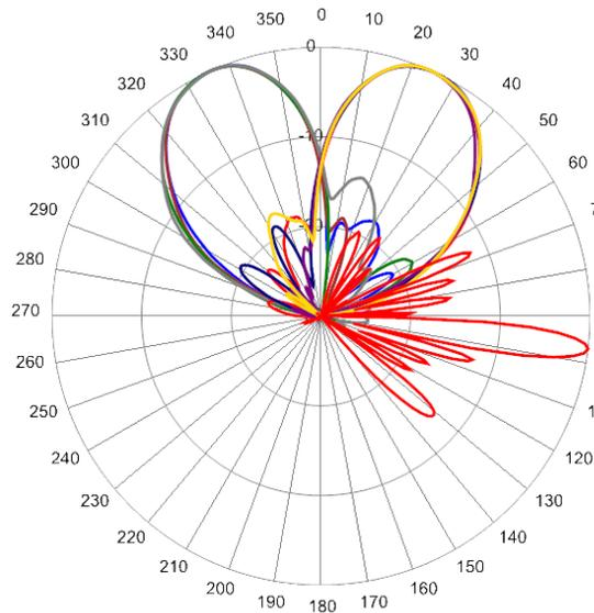
2340 MHz Azimuth with Elevation 7°
