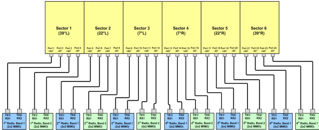
MBM Series "U Band" Multisector Antenna (2x2\_Two Band Connection)
