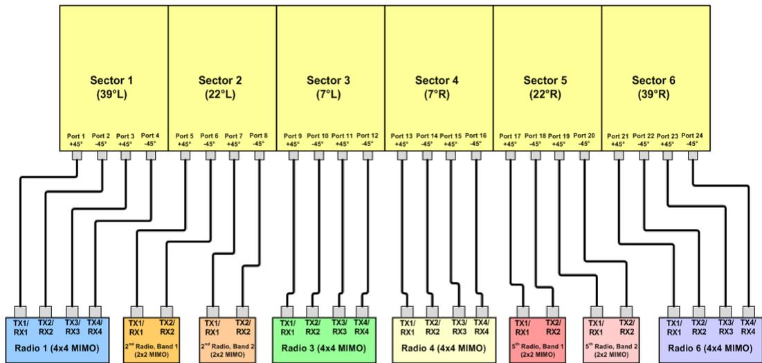
MBM Series "U Band" Multisector Antenna (4x4\_and\_2x2 Mixed Connection)
