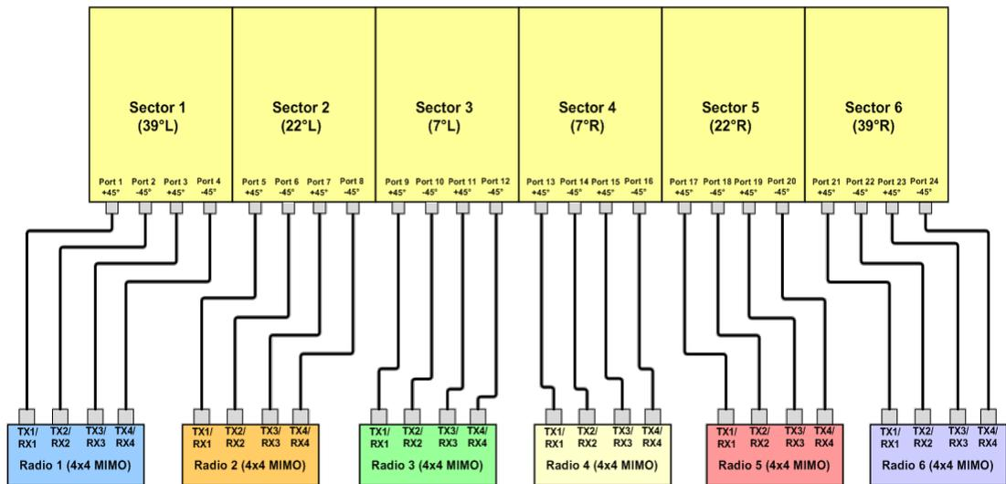
MBM Series "U Band" Multisector Antenna (4x4 Connection)
