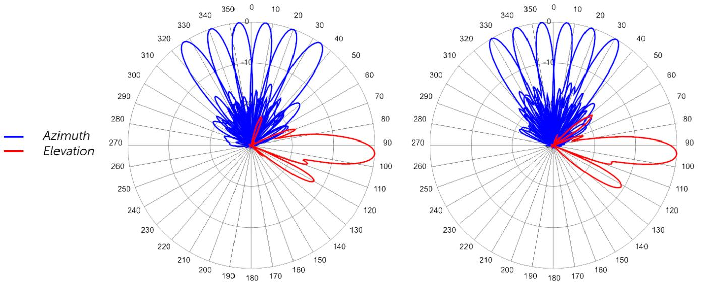
2170 MHz Azimuths with Elevation 4°
