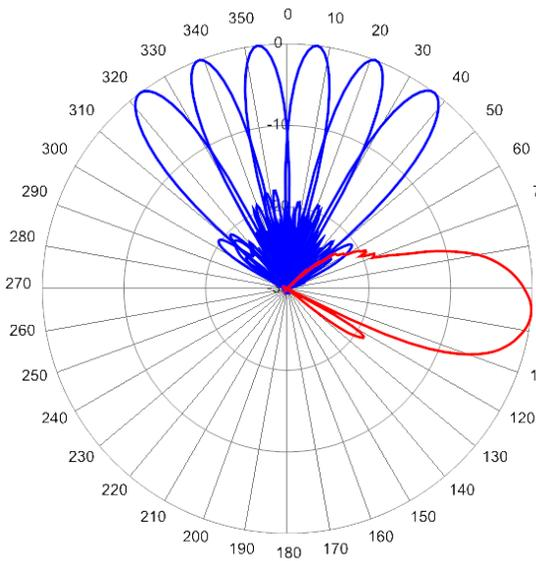
2310 MHz Azimuths with Elevation 6°
