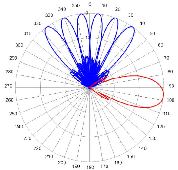
2355 MHz Azimuths with Elevation 6°
