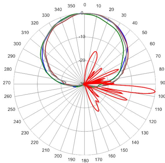
2340 MHz Azimuth with Elevation 6°
