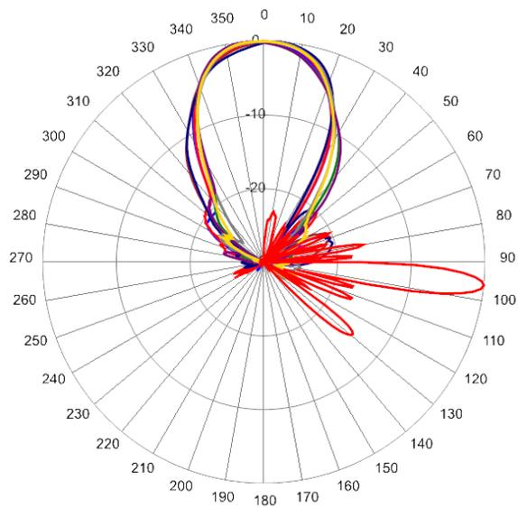
2340 MHz Azimuth with Elevation 6°
