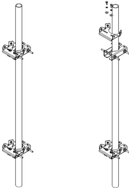
**Fig. 4: Dual Hinge Bracket Mounting to Clamps**
