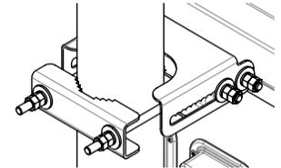
Fig. 4: Fixed Mast Bracket
