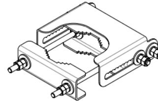
Fig. 3: Installed Adjustable Bracket
