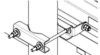
Fig. 6: Detail Of Adjustable Tilt Bracket
