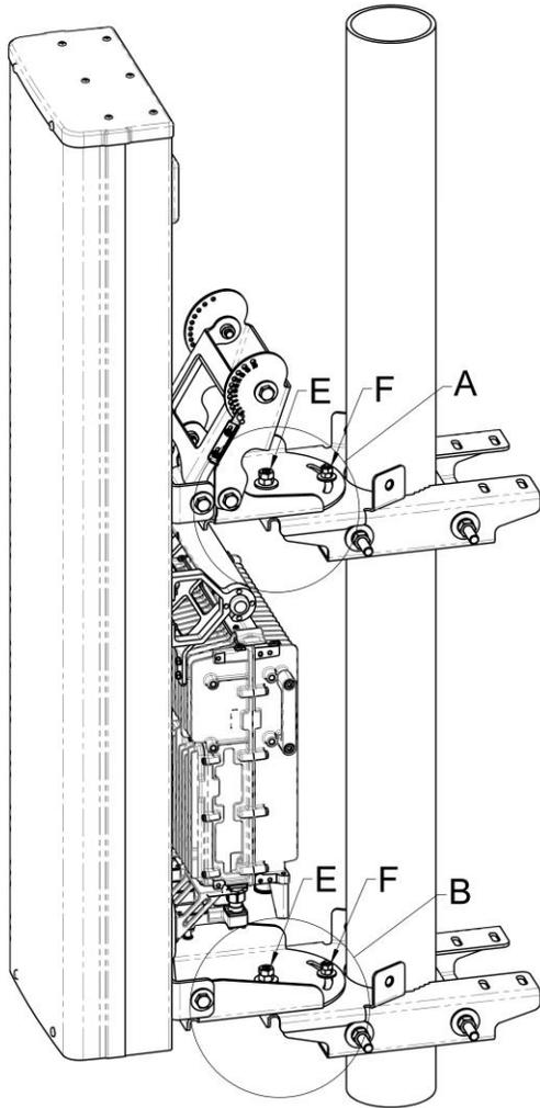
Fig. 20: Swivel Adjustment (Detail A and Detail B)
