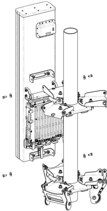
**Fig.14: Installation of Antenna on Fixed and Adjustable Brackets – Uptilt Setup (Side View)**
