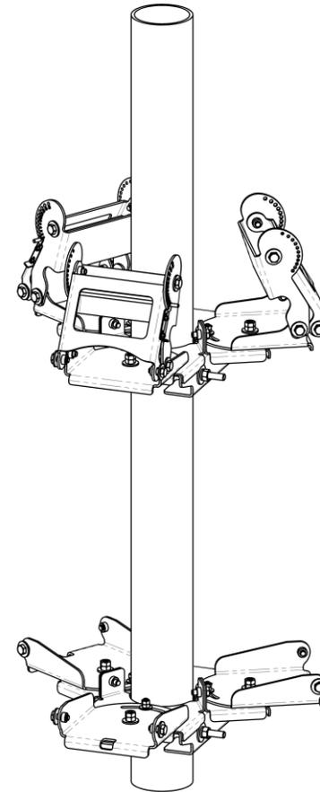
**Fig.7: Installation of 1<sup>st</sup> Antenna/Radio Assembly on Fixed and Adjustable Triple Mount Brackets – Downtilt Setup (ISO View)**
