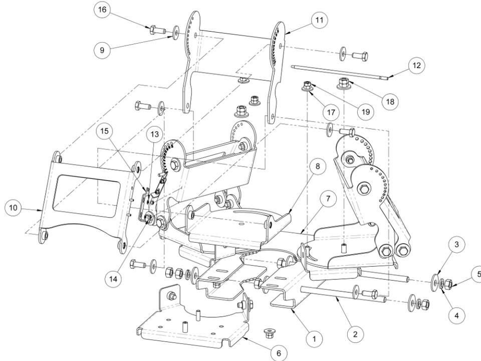
**Fig. 2: Swiveling Triple MDT Adjustable Bracket BOM**
