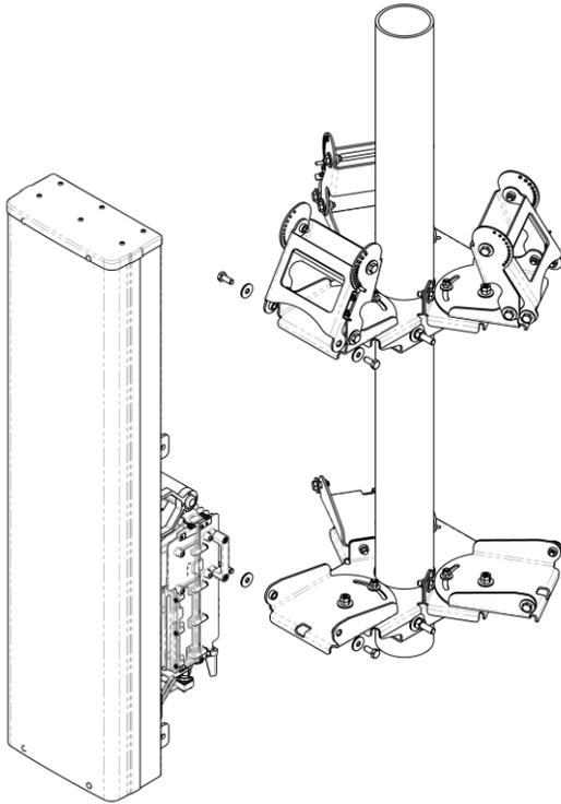
**Fig.8: Installation of 1<sup>st</sup> Antenna/Radio Assembly on Fixed and Adjustable Triple Mount Brackets – Downtilt Setup (Side View)**
