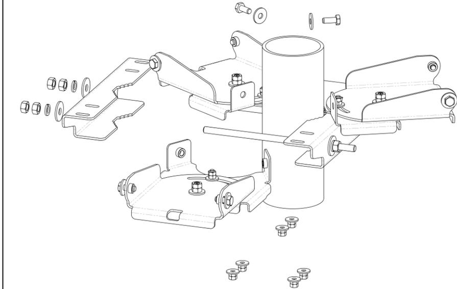
**Fig. 4: Adjustable Triple Bracket Mounting on Mast**
