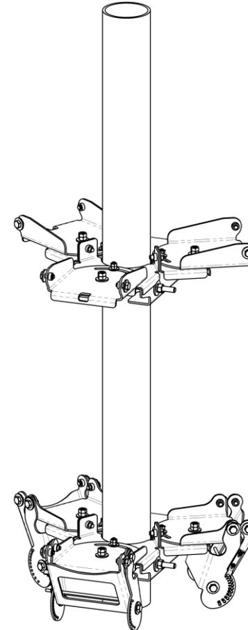
**Fig.13: Installation of Antenna on Fixed and Adjustable Brackets – Uptilt Setup (ISO View)**
