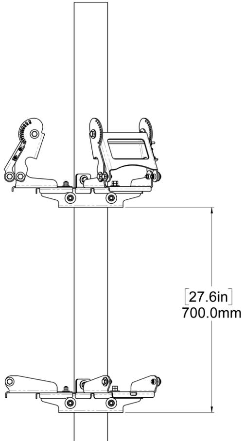
Fig. 6: Orientation of Fixed and Adjustable Triple Mount Brackets – Downtilt Setup
