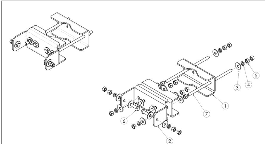
**Fig. 1: Fixed Mast Bracket Kit BOM**
