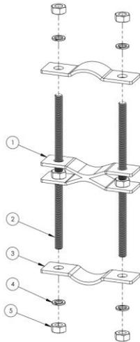
**Fig. 1: MBC-10 Mast Bracket Clamp BOM**
