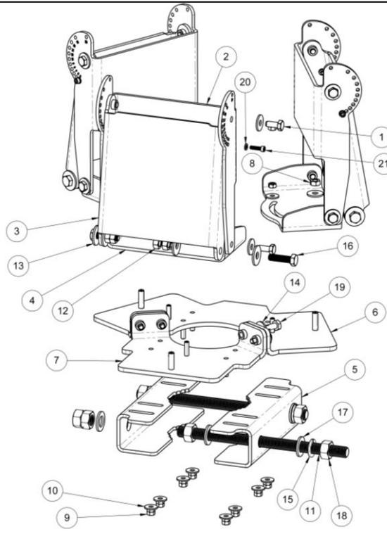
**Figure 2: Triple Swiveling Mechanical Tilt (MT) Adjustable Bracket BOM**
