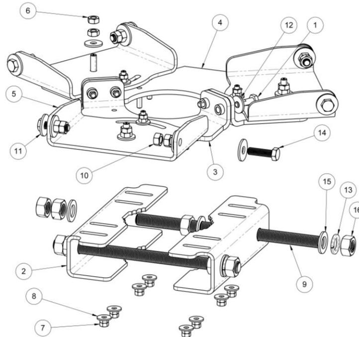
**Figure 1: Triple Swiveling Mechanical Tilt (MT) Fixed Bracket BOM**
