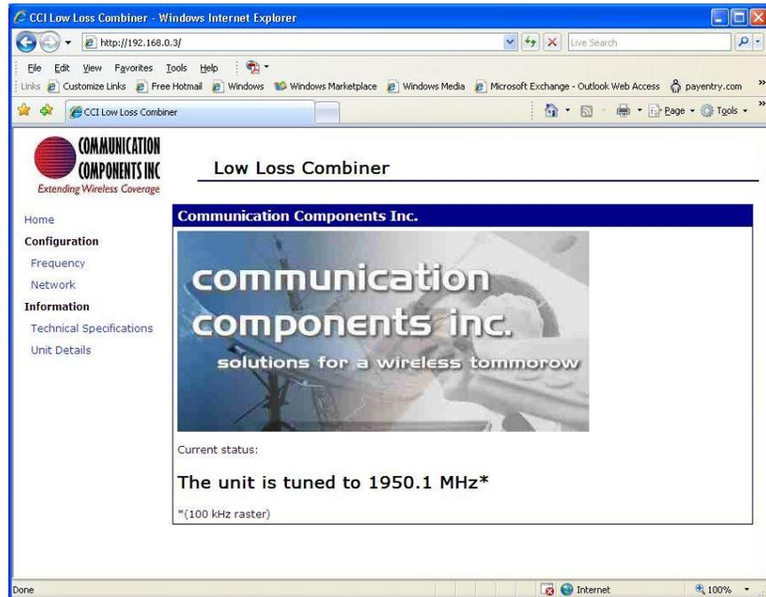
Figure 5.18 – Browser screen indicating completion of “Enter Frequency” tuning process
