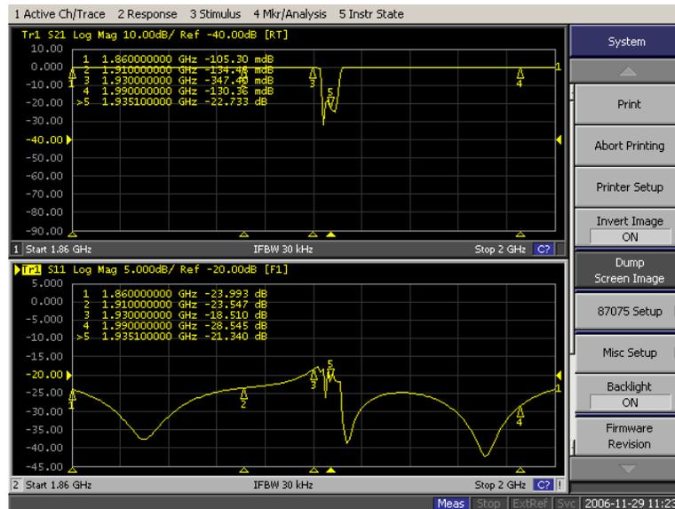
Figure 5.20 – Analyzer response when viewing the “2G” (GSM) port (UMTS frequency tuned to 1935.1 MHz)
