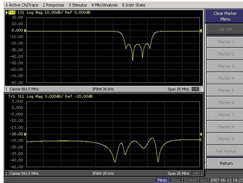
**Figure 5.20 – Analyzer response when viewing the GSM port (UMTS frequency tuned to 885.1 MHz)**
