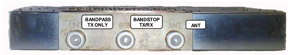
Figure 5.2 – Rear Panel RF showing RF Connections
