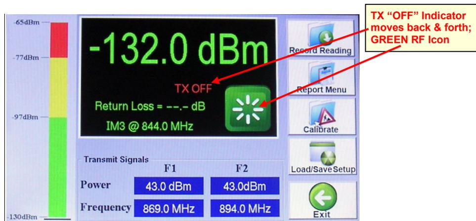
**Figure 20 - PIM and Return Loss Window with "TX OFF"**
