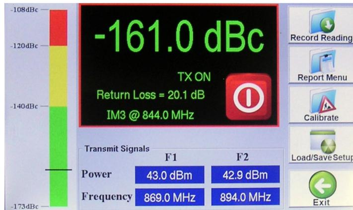
Figure 40 - **PIM and Return Loss** Window during “TX ON” (Reading in dBc)
