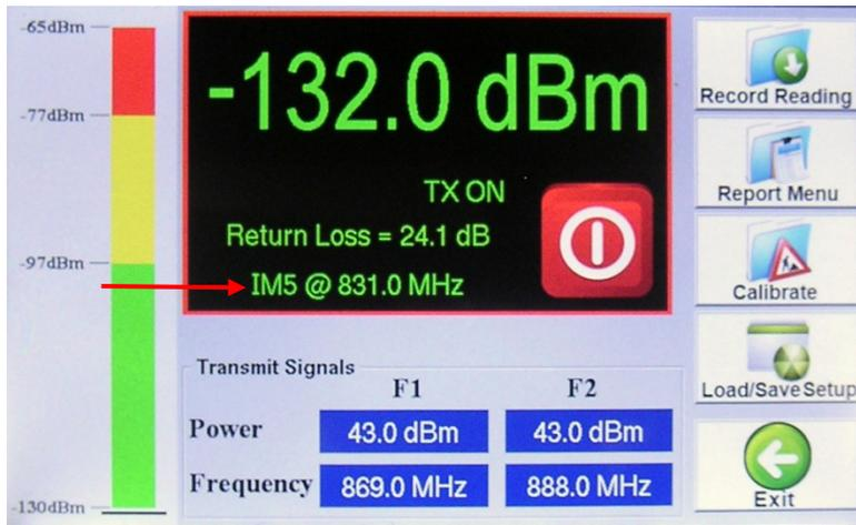
**Figure 46 - *PIM and Return Loss* Measurement Window when Set for IM5 Readings**
