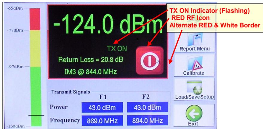
**Figure 24 – PIM and Return Loss Window with “TX ON”**
