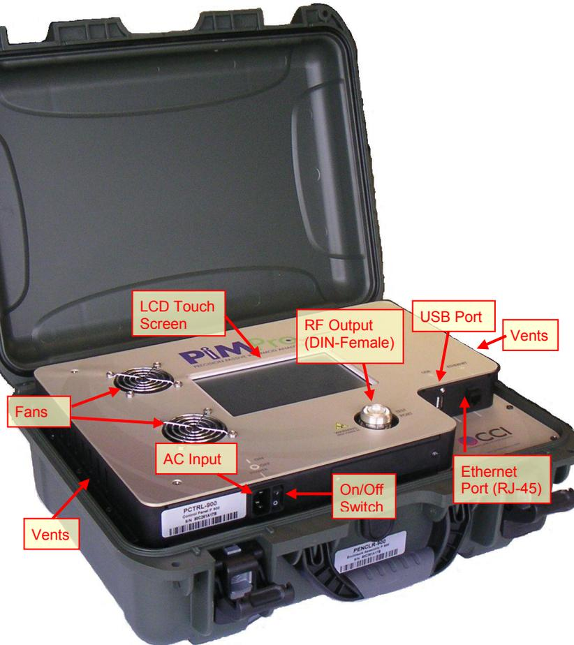
**Figure 12 - Overall view of the CCI PiMPro PIM Analyzer**
