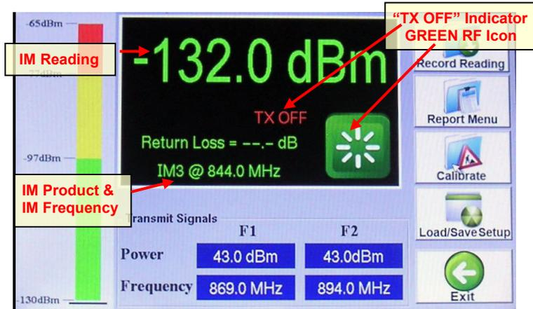
Figure 39 - **PIM and Return Loss** Window during “TX OFF” (Reading in dBm)
