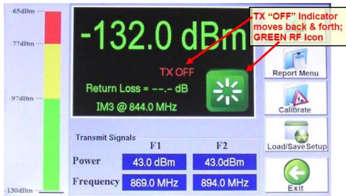
**Figure 4 - *PIM and Return Loss* Screen with “TX OFF”**
