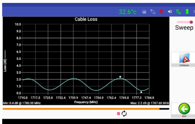
Figure 45 – Cable Loss Measurement
