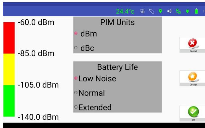
**Figure 17 - *Configure PIM Scale* Window**
