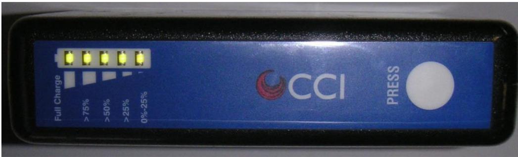
**Figure 69 – Fully Charged Battery LED Status Indicators**
