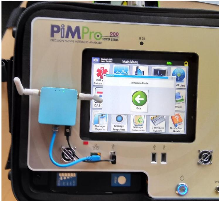
**Figure 1 – Wireless Router Mounted on PiMPro**
