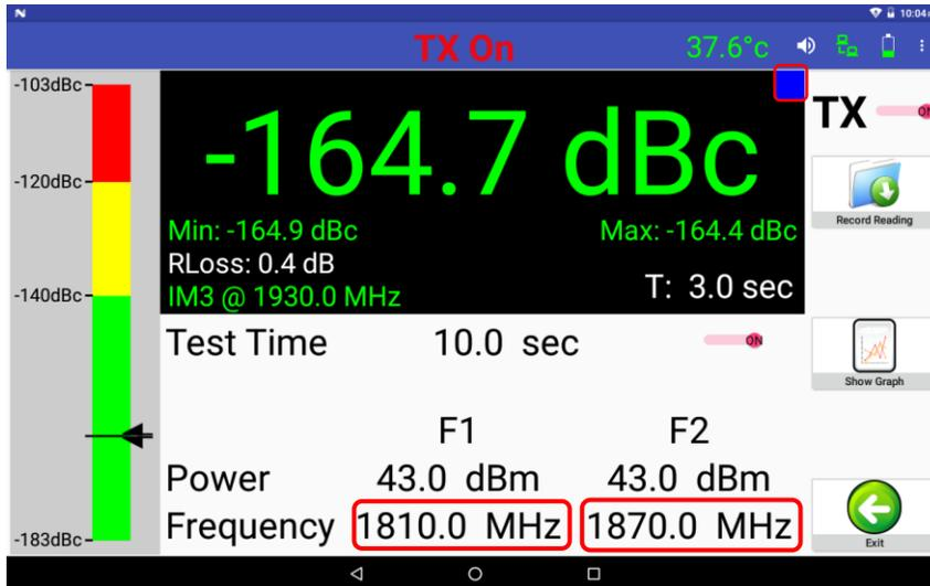
**Figure 9 – PIM & R.Loss Screen Prior to Test**
