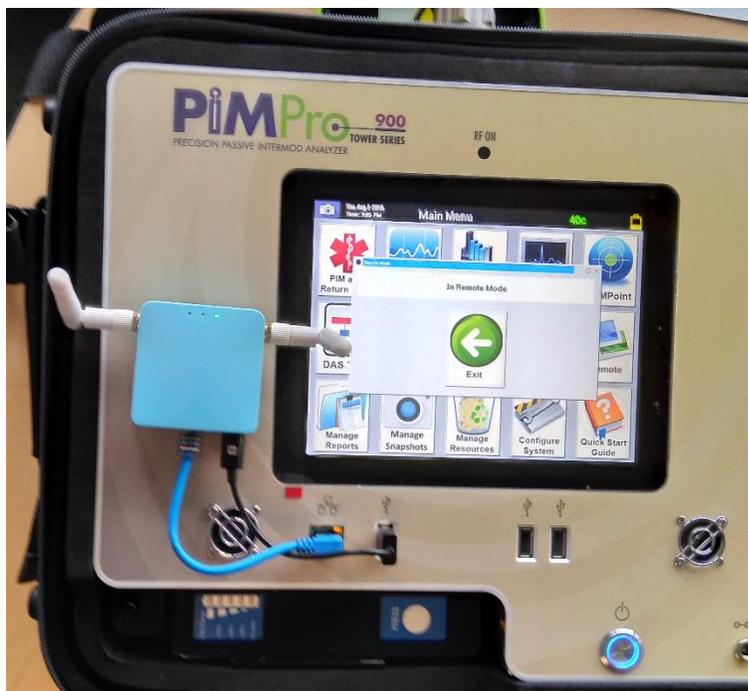
**Figure 131 – Wireless Router Mounted on PiMPro**
