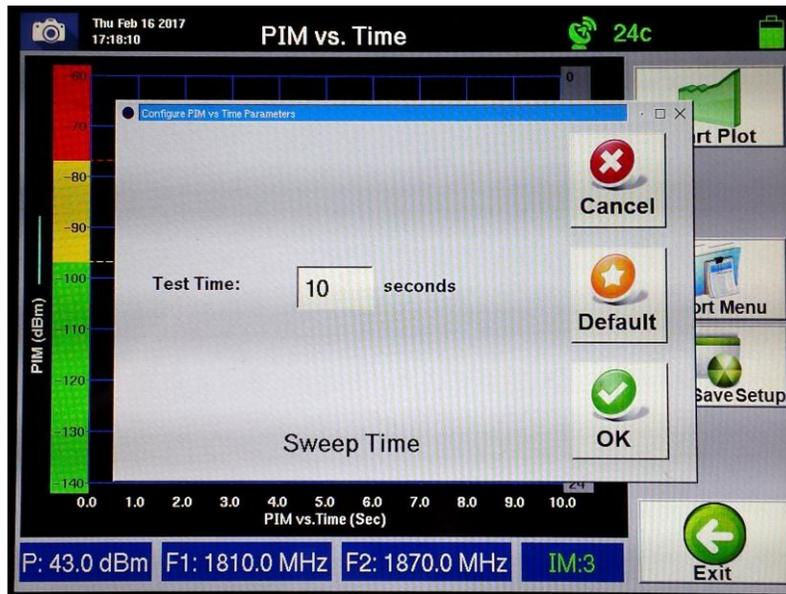
**Figure 53 - *Configure PIM vs. Time Parameters* Window**
