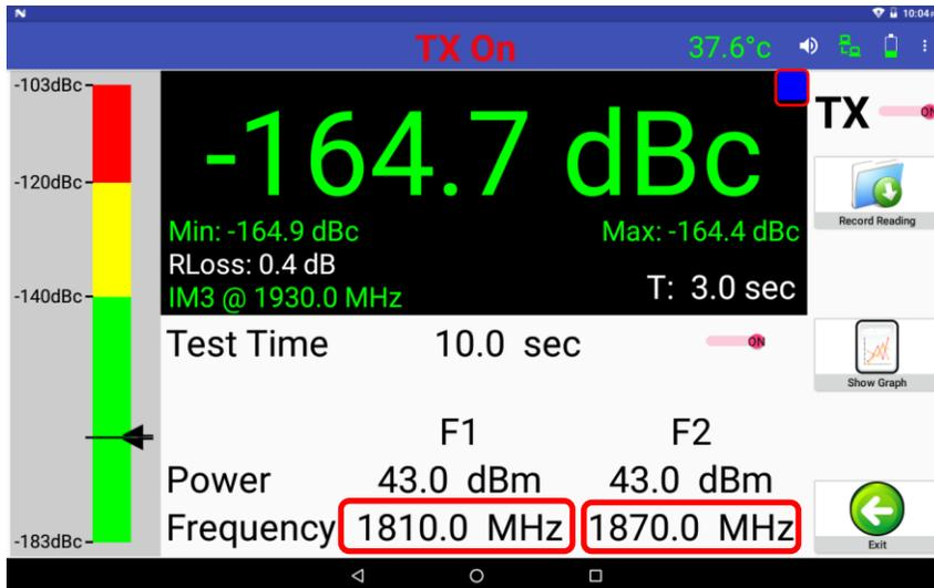
**Figure 139 – PIM & R.Loss Screen Prior to Test**
