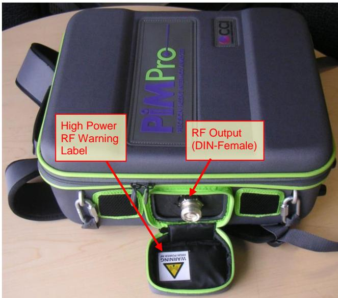
**Figure 13 – Tower Series RF Output Port**
