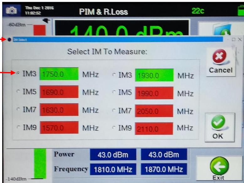
**Figure 49 - *IM Select* Window for (IM3) @ Standard F1 = 1810.0 MHz and F2 = 1870.0 MHz**
