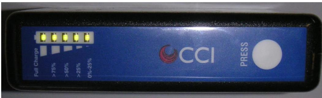
Figure 168 – Fully Charged Battery LED Status Indicators
