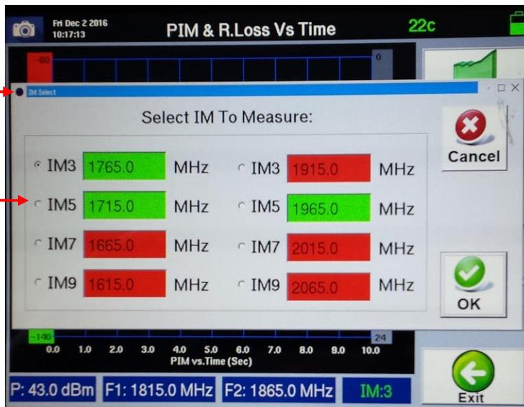
**Figure 50 - *IM Select* Window for IM5 at F1 = 1815.0 MHz and F2 = 1865.0 MHz**
